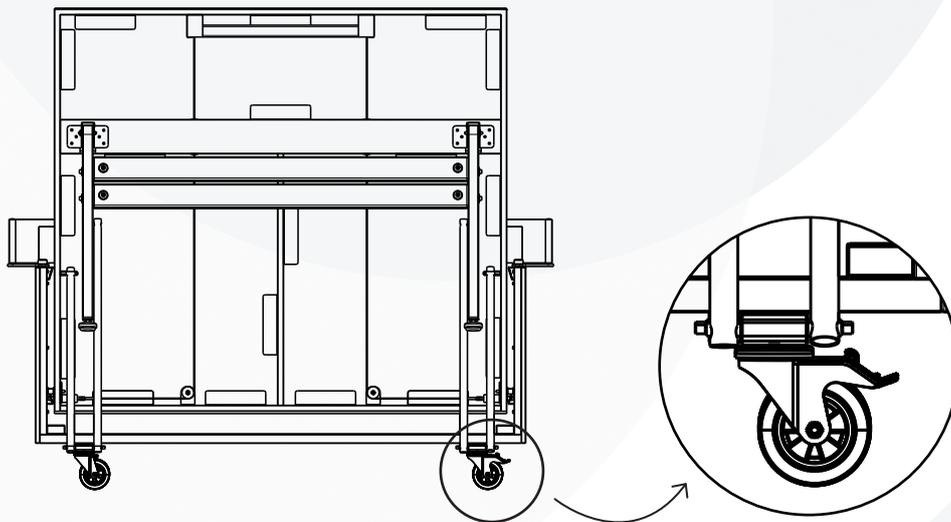
**Brake the wheels pressing the pedal.**
