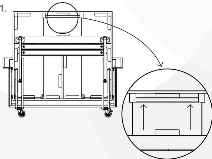
Press up the wooden piece located at the back side of the ping pong table to unlock it.
