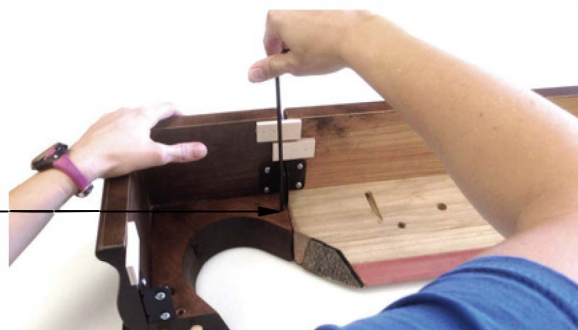
ACCESS HOLE FOR RAIL LOCK FASTENER
