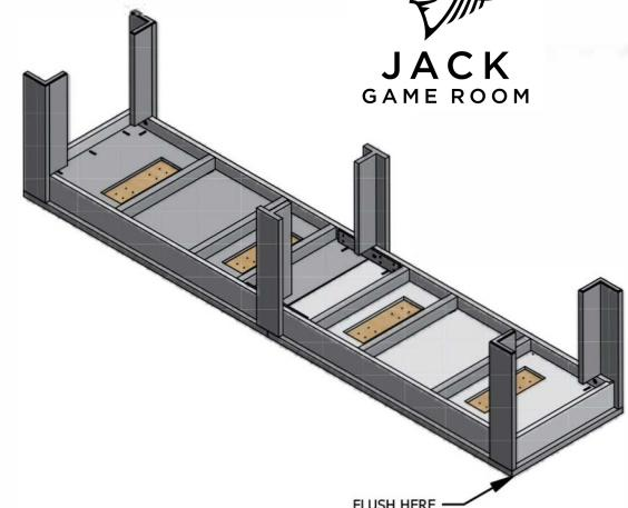
**3** PLACE THE LEGS IN POSITION AND FASTEN THE LEGS TO THE CRADLE USING THE BOLTS PROVIDED. BEFORE TIGHTENING THE BOLTS, ADJUST THE POSITION OF THE END LEGS SO THAT THEY ARE FLUSH WITH THE END OF THE TABLE TOP RAIL.
