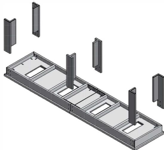
**2** IDENTIFY THE PAIRED END LEGS (LEFTS AND RIGHTS) AND CENTER LEGS. THEY WILL BE INSTALLED ON THE TABLE AS SHOWN.
