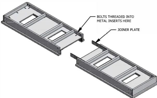
**1** PLACE THE CRADLE HALVES IN POSITION IN YOUR ROOM AND LAY THEM UPSIDE-DOWN ON A PROTECTIVE SURFACE SO THAT NO DAMAGE IS DONE TO YOUR FLOOR OR TO THE CRADLE. FASTEN THE TWO HALVES TOGETHER USING THE JOINER PLATE AND THE BOLTS PROVIDED.
