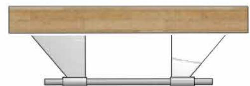
**6** ADJUST THE CLIMATIC ADJUSTERS SO THAT THE PLAYFIELD IS SLIGHTLY CONCAVE (THE MIDDLE OF THE TABLE BOWS DOWNWARD). USE THE OUTER AND INNER NUTS TO MAKE ADJUSTMENTS TO THE CONCAVITY OF THE PLAYFIELD.
