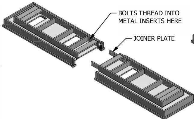
**1** PLACE THE CRADLE HALVES IN POSITION IN YOUR ROOM AND LAY THEM UPSIDE-DOWN ON A PROTECTIVE SURFACE SO THAT NO DAMAGE IS DONE TO YOUR FLOOR OR TO THE CRADLE. FASTEN THE TWO HALVES TOGETHER USING THE JOINER PLATE AND THE BOLTS PROVIDED.
