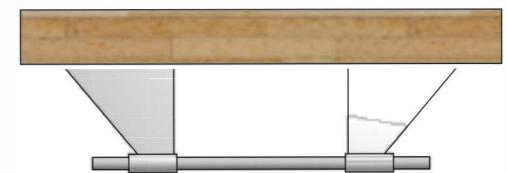
**6** ADJUST THE CLIMATIC ADJUSTERS SO THAT THE PLAYFIELD IS SLIGHTLY CONCAVE (THE MIDDLE OF THE TABLE BOWS DOWNWARD). USE THE OUTER AND INNER NUTS TO MAKE ADJUSTMENTS TO THE CONCAVITY OF THE PLAYFIELD.
