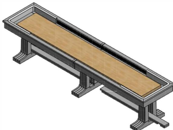
**4** INSTALL THE STRETCHERS BY SLIDING THEM THROUGH THE CENTER OF THE LEGS TOWARD THE CENTER OF THE TABLE. THEY SIMPLE REST IN PLACE ON TOP OF PRE-INSTALLED BLOCKS ON THE LEGS. VELCRO STRAPS KEEP THE STRETCHER IN PLACE. NO HARDWARE IS REQUIRED.
