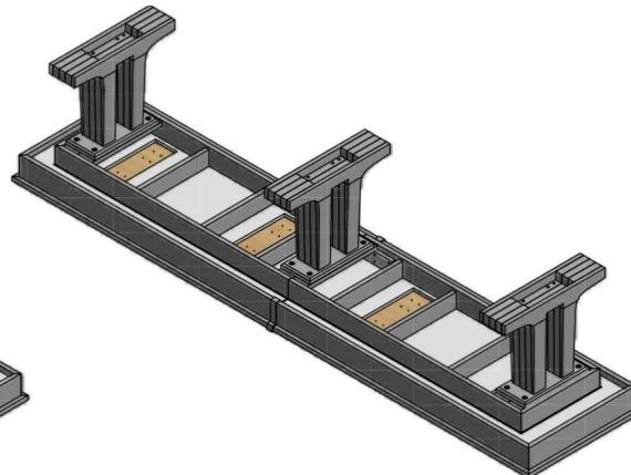
**2** PLACE THE LEGS IN POSITION AND FASTEN TO THE CRADLE USING THE BOLTS PROVIDED.
