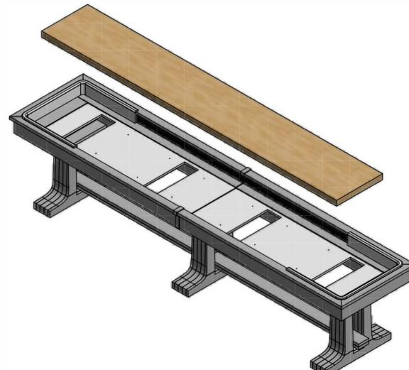
**5** SET TWO SHUFFLEBOARD PUCKS ON EITHER END OF THE TABLE, THEN GET HELP TO LIFT THE PLAYFIELD INTO THE CRADLE, ON TOP OF THE PUCKS. FROM UNDERNEATH THE TABLE, LIFT THE PLAYFIELD AND REMOVE THE PUCKS. LEVEL THE TABLE USING THE ADJUSTABLE LEVELS ON THE LEG.
